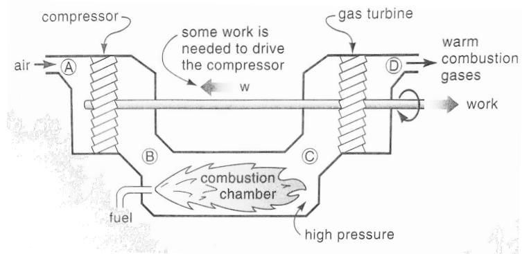
Advantage over the Rankine cycle: no need for a heat exchange network.
